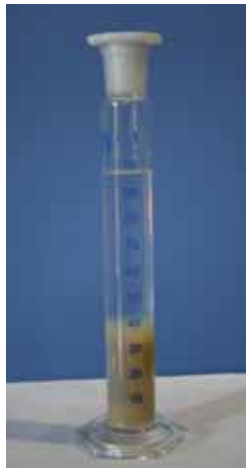
2 gr sodium bentonite swell minimum 24 ml in pure water.
